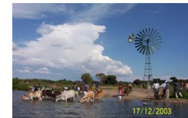
24ft Kijito Windpump pumping water from Lake Victoria near Musoma Tanzania for lakeside irrigation (UNDP Irrigation Project)
