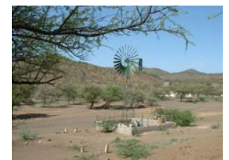
24ft Kijito Windpump pumping water from Lake Victoria near Musoma Tanzania for lakeside irrigation (UNDP Irrigation Project)
