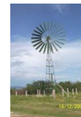
24ft Kijito Windpump pumping water from Lake Victoria near Musoma Tanzania for lakeside irrigation (UNDP Irrigation Project)
